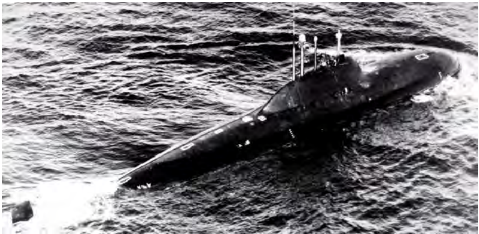
The fastest reactor? – A “ЛЯРА” (Alfa) class submarine (1969-81) was powered by a 155 MW fast reactor and could achieve a speed of 76 kph.
